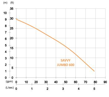
Shaft Speed: 2850 rpm Outlet: 50mm, 2in
